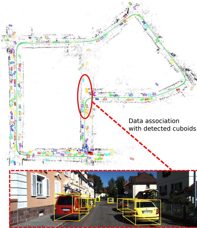
Fig. 7: Mapping result (top view) for the KITTI odometry sequence 07. In addition to the black map points and green KeyFrames, detected cars are rendered as colored rectangles. 7 colors are repeatedly used to tint the cuboid for better visualization. A KeyFrame is selected to demonstrate the data association between cuboid observations and existing objects.
